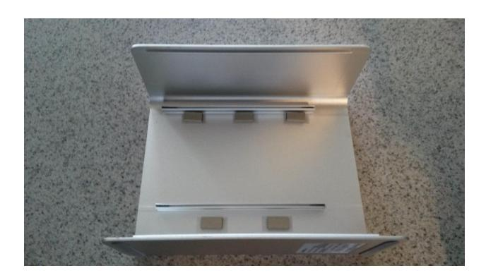
8. Remove the 4 short screws holding the inner metal frame together:
